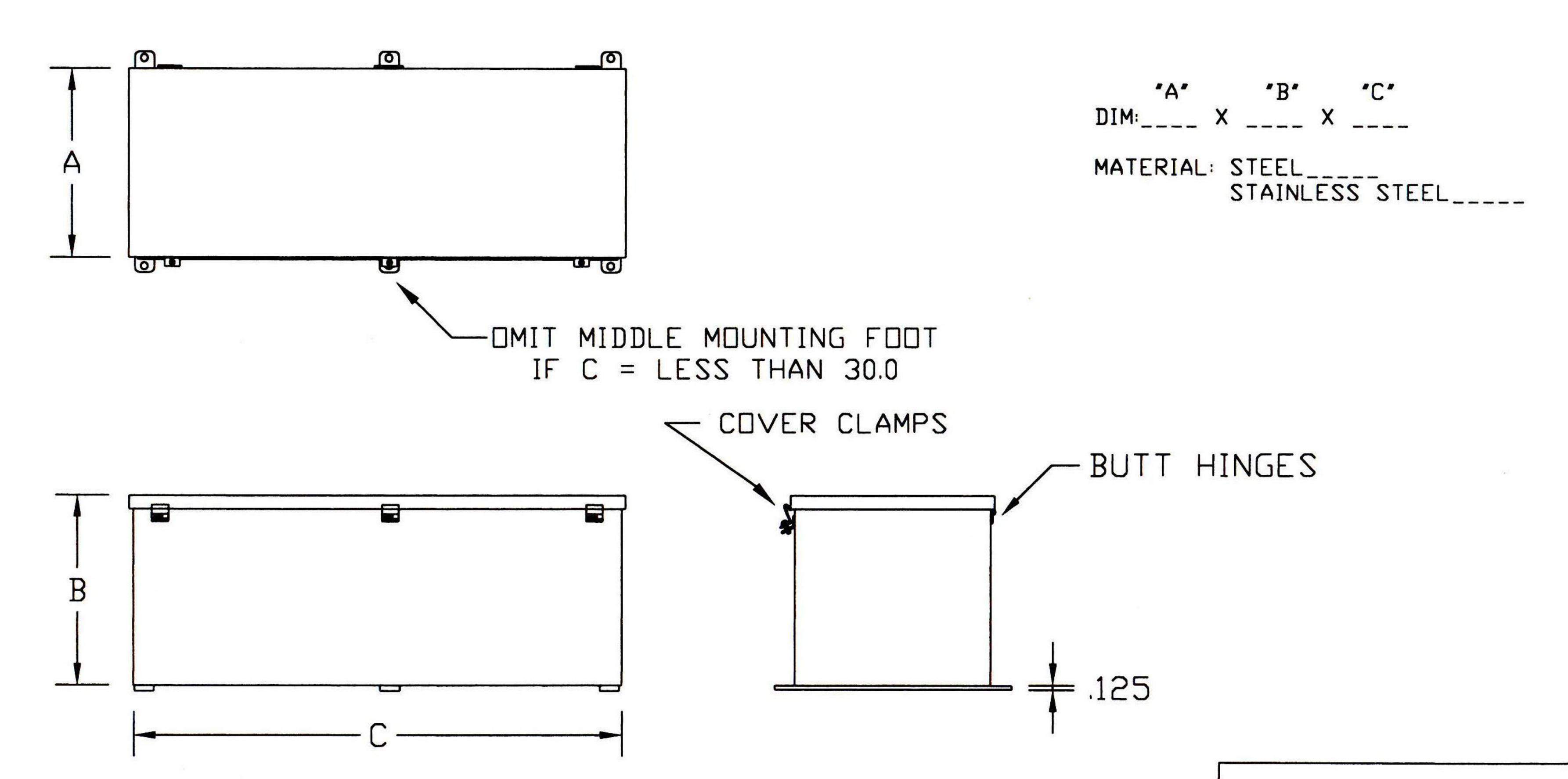
NOTES: MADE FROM 14GA. SHEET STEEL WELDED SEAMS, GASKETED COVER
